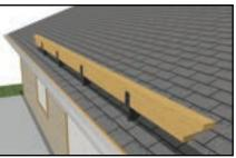
Each *LO-PRO* Patio Roof Riser will come with the bolts for securing the beam, however, you can also use (12) Simpson **1/4**" **x 1-1/2**" SDS screws per bracket instead.
