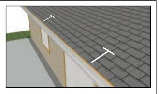
Note: If you have closed soffits, the easiest way to locate your rafters is by lifting your roofing material and looking for a plywood joint. This should tell you exactly where your rafter is located.
