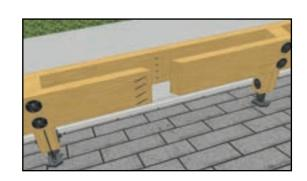
The diagonal cut is to prevent light from passing through the joint and typically cut at ~30°. The screws are installed on the back side of beam for concealment.
