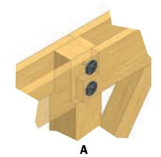
On the ground side, this joint must always be sitting on top of a beam or a notch. Depicted to the right (A) is an example of double 2x8 beams, notched so they can be secured with two through bolts and bridge washers. The other image (B) shows two 4x8s butt together and secured with a T-brace.
