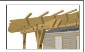
First, we measure down **1-1/2**" from the top of our beam/rafter and up **1-1/2**" from the bottom and make a line along the length of the board. The angle that you choose for the diagonal cut can be whatever you'd like. We typically make it ~**35**°. Make your cuts with a skill saw and finish with a jig saw.
