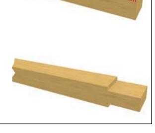
You can also create a notch for a single 4x8 beam on a 6x6 post instead of using a 4x6 post and a T-brace as depicted on the previous page.
