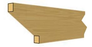
Making the cut like this on a 4x8 beam can prove more tricky, so we will usually measure **3**" from the top instead and cut the angle all the way to the bottom of the board with a beam saw.
